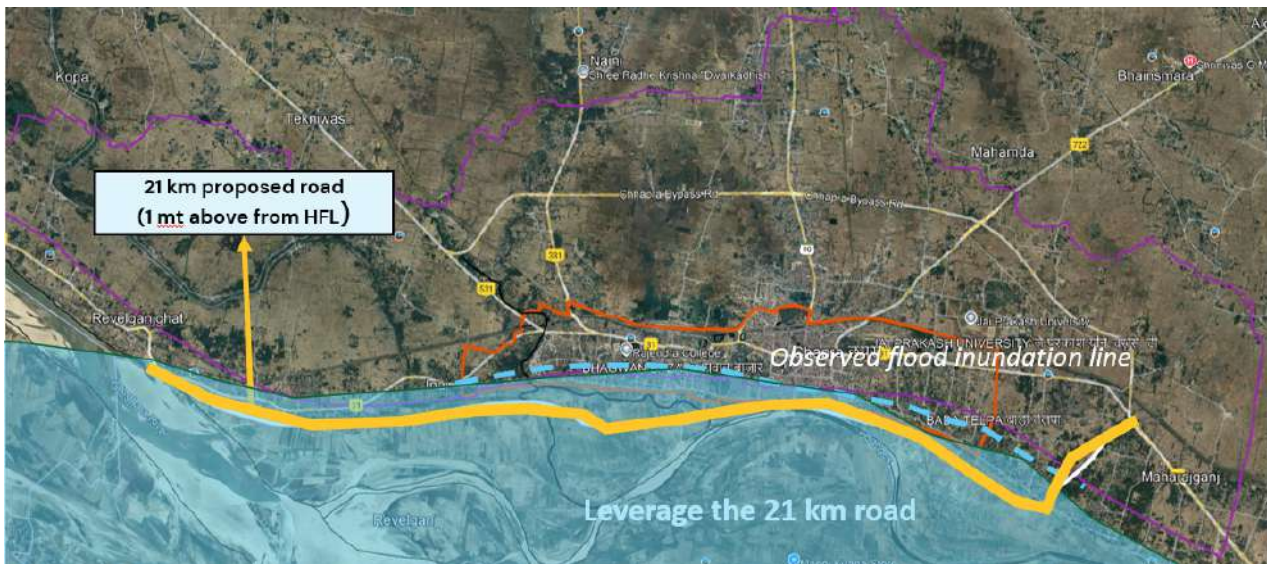
Figure 12: Map displaying the alignment of the proposed 21 km road in Chapra
